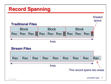
This diagram shows the difference in record and block structures for traditional and stream files.
